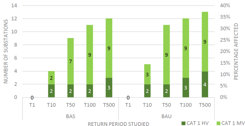
Figure 41. Number of affected substations in the current (BAS) and future (BAU) scenarios and their percentage over the total number of substations located in Barcelona.
